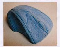
Educantage of using blue modelling. Soamis it is easely mould end Cut and shope of the Disadvantage is that it you can't remouldit to change the shope you have to Start dequin
